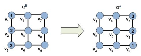
**Solution** of an instance of cooperative path-finding on a graph with R={1,2,3}
